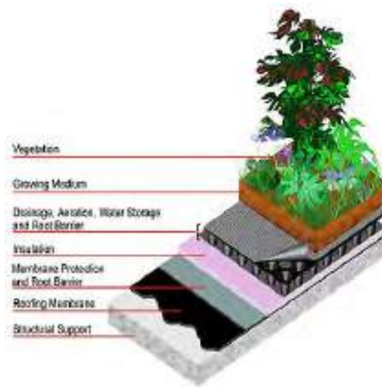
Figure 8-12. Vegetated Roof Cross-Section
