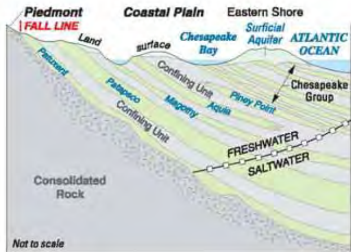
The Northern Atlantic Coastal Plain Aquifer System Source: A Science Plan for a Comprehensive Regional Assessment of the Atlantic Coastal Plain Aquifer System
